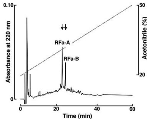
FIG. 1. HPLC of an adsorbed fraction from an immunoaffinity column on a reverse-phase ODS-120T column ( $0.46 \times 25$  cm;  $10\text{-}\mu\text{m}$  particle size) at a temperature of  $40^\circ\text{C}$  and a flow rate of  $1\text{ ml/min}$ . The dashed line represents a gradient of acetonitrile in  $0.1\%$  TFA. Arrows indicate elution positions of synthetic RFa-A and -B.
