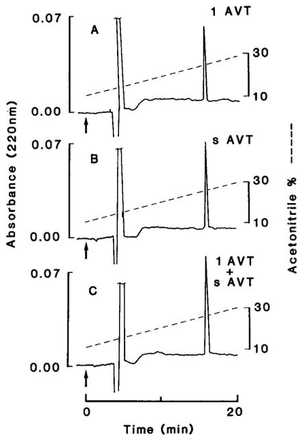
FIG. 2. Comparison of the RP-HPLC elution positions of lamprey AVT (A), Chum salmon AVT (B), and a 1:1 mix of lamprey and salmon preparations (C). RP-HPLC under identical conditions, as described in the text. Arrows, time of injection.
